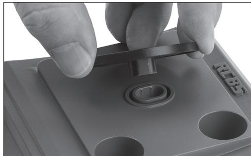
Photo 5: Insert platen into load cell pocket
