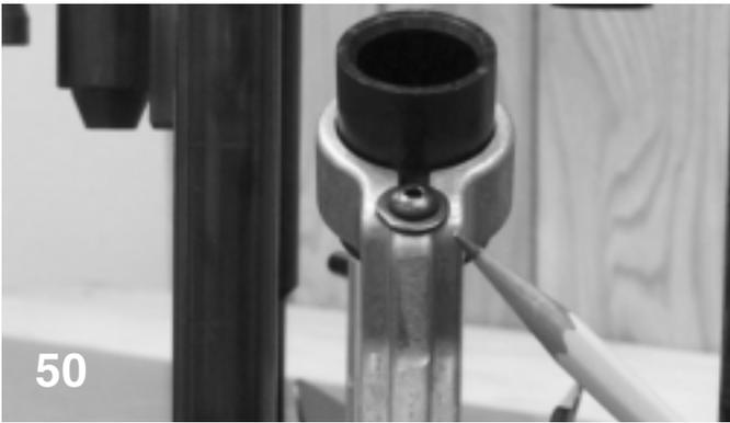
**15. Wads crush hull mouths upon insertion:**
