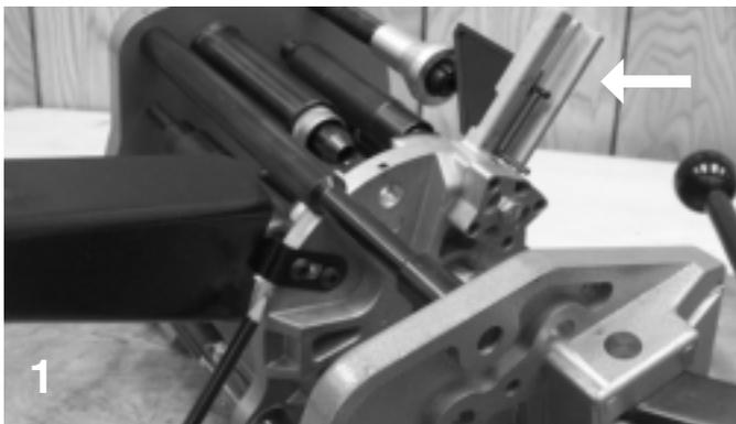
After laying press on bench, remove plastic tie securing the Lockout pin to the Ram of the press and remove Lockout pin. (photo 2) The Lockout pin can be used with a small lock (not included), to secure press when not in use.
