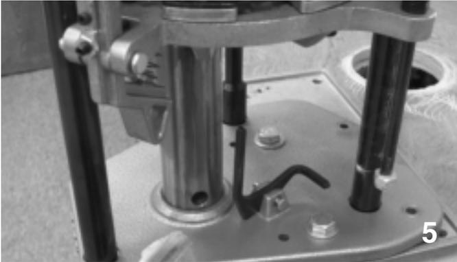
Select an area on your bench with approximately one-foot clearance on each side of The Grand. Install press with three 3/8" bolts or four 1/4" bolts, length to be determined by the thickness of your bench (mounting hardware not included). The press can also be mounted on our optional Riser Stand, which raises the press four inches above your bench (Riser Stand part number 89010) (see photo 6).
