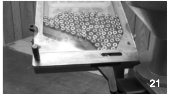
Primer is dropped from the Primer Drop Tube Collet to the Primer Transfer Bar (*photo 22*).
