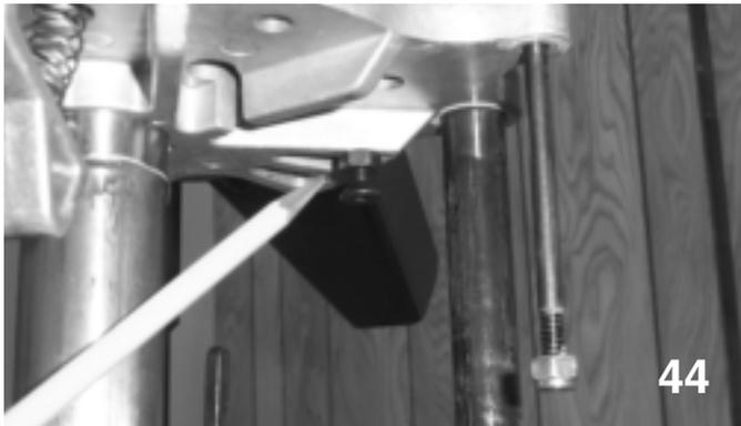
3. Adjusting the upper bushing of the size die will increase or decrease the amount force used to push the hull from the Size Die. Adjust so you feel the minimal amount of force to size but enough to eject the spent primer and push the hull from the Size Ring. (see photo 45.)
