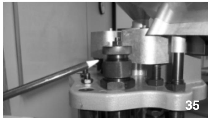
3. **Priming Station Adjustment** The Primer Stem Assembly is under spring tension to compensate for varying internal base wad heights between hull manufacturers. Should it become necessary to adjust primer depth, the Primer Seater Body Assembly can be moved up or down. To make this adjustment, loosen the top 3/4" lock nut and screw rod up or down in 1/4 turn increments until desired primer seating depth is achieved (*photo 36*).
