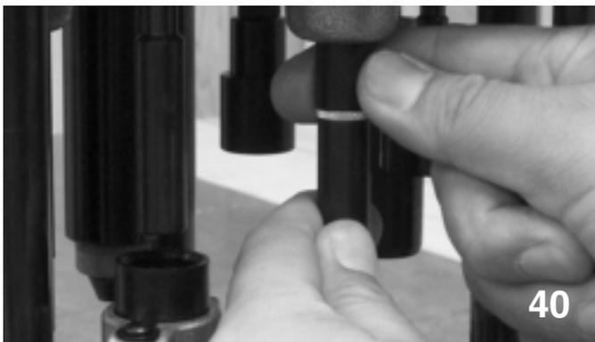
7. **Crimp Start Adjustment** Crimp start is an up or down adjustment. Loosen the top lock nut (A) and adjust Crimp Start assembly up or down, retighten lock nut (*photo 41*). Too much Crimp Start can cause a bulge on the side at the top of the hull during crimp. Not enough crimp start can leave a hole in the center of your hull after crimp.
