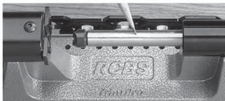
*Lubricate the case trimmer shaft.*
