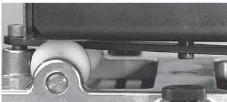
*Lubricate the roll pin on the bottom of the motor housing.*
