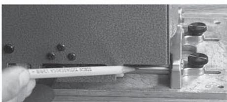
*Lubricate the guide rods.*
