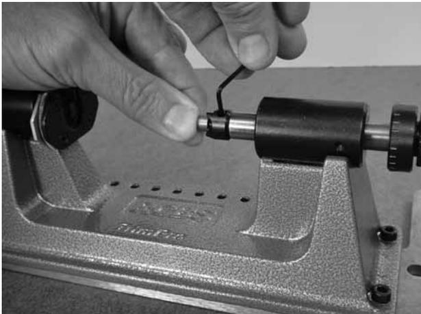
**Photo 6. Installing Pilot**
