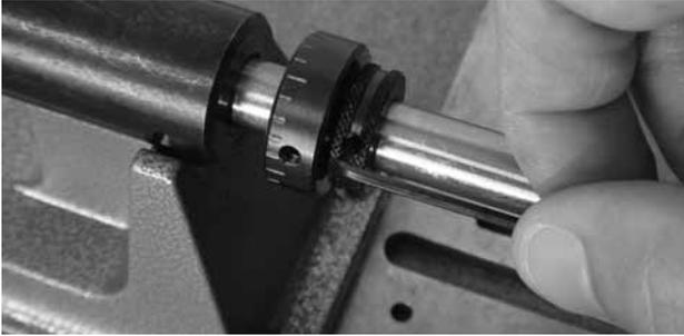
**Photo 17. Coarse Adjustment Bushing**
