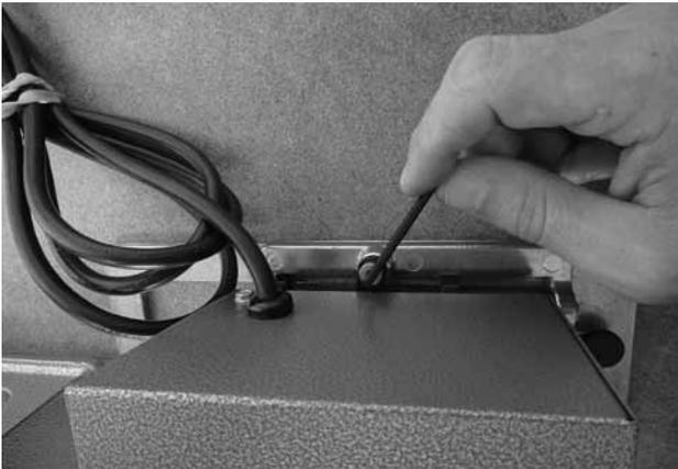
**Photo 4. Install Shoulder Bolt**
