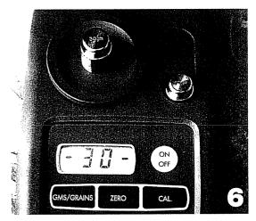
Press CAL. After displaying "HOLD" the scale will ask you for 50 grams. Add the 20 gram weight to the top of 30 gram weight already on the platform. NOTE: At this point BOTH weights must be on the platen. See Photo 7.
