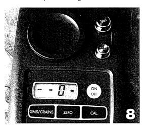
Remove both check weights and press CAL for the last time. The scale will read zero.
