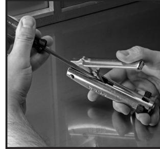
Photo 7: Centering Internal Linkage
