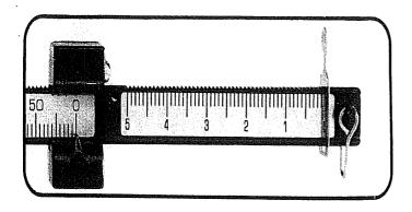
To increase weight values, move the poise to the left and line it up with the desired graduation. Always make sure the pawl is seated in the notch.
