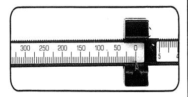
To increase weight values, move the poise to the left and line up the indicator with the desired graduation. Always make sure the pawl is seated in the notch.
