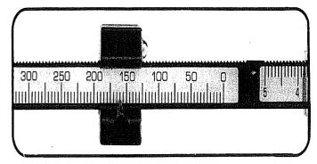
Do not attempt to set the large poise at any position except firmly seated in a notch. Always use the smaller poise for weight values between the 5 grain increments of the large poise.
