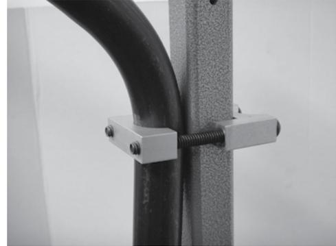
**Photo 18. RCBS Tube require square side of Clamp**
