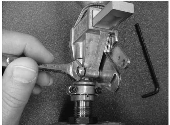
**Photo 2. PM Bellcrank Locknut**
