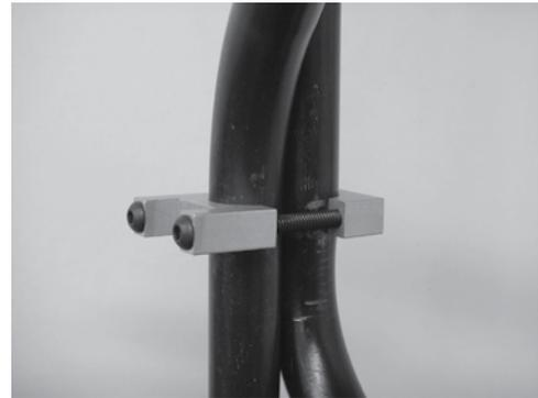
**Photo 19. Dillon Tube require round side of Clamp**
