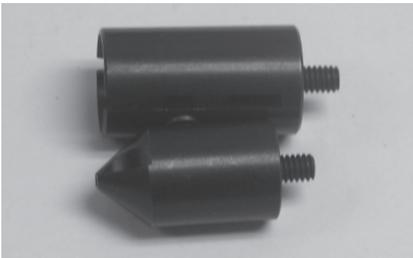
Photo 6: Outside Deburr & Inside Chamfer Tools
