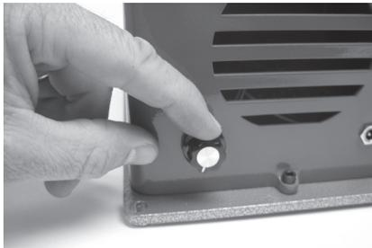
Photo 8: On/Off/Speed Control in OFF Position
